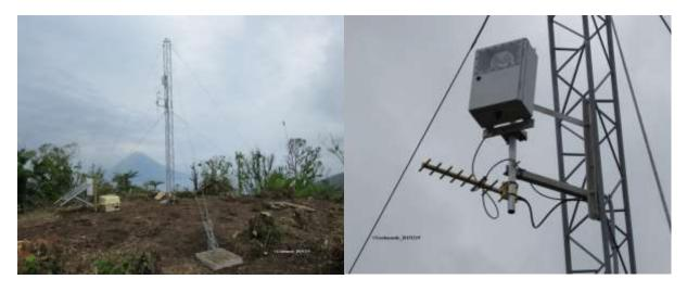
Figure : The complete setup of tower on Paama islands and the Webcam pointing to Lopevi for visual monitoring. It was built in the month of December from 15th to 21th
