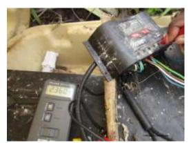
Over discharge of batteries
