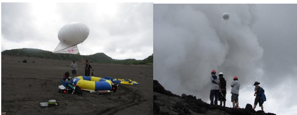
Balloon deployment on yasur tanna, July 2017: The Balloon is filled with hydrogen. Geophones are attach on the balloon and measured explosions came out from Yasur Volcano
