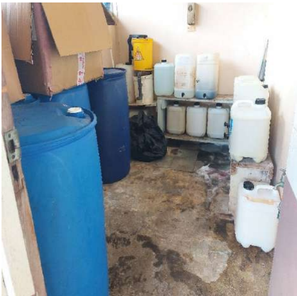
Fig. 4.9 Poor chemicals storage practices
