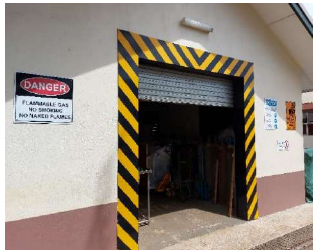
Fig. 4.6 Good chemical labelling practices at work places
