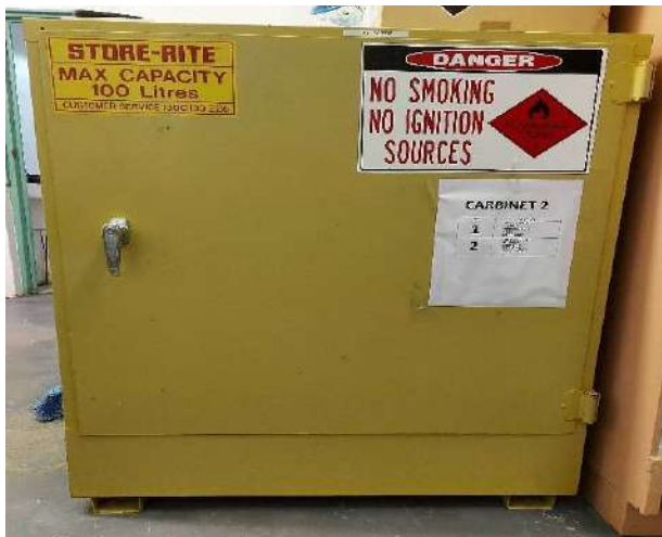
Fig. 4.6 Good chemical labelling practices at work places
